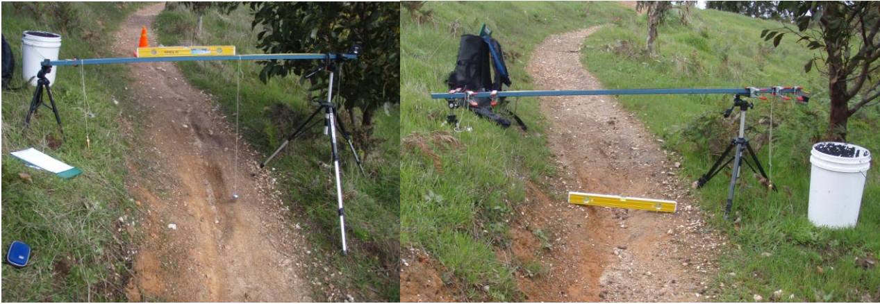
Figure 21 Dynamic Tension transect point #1 in September 2008 and September 2009 showing the widening of the riding channel
