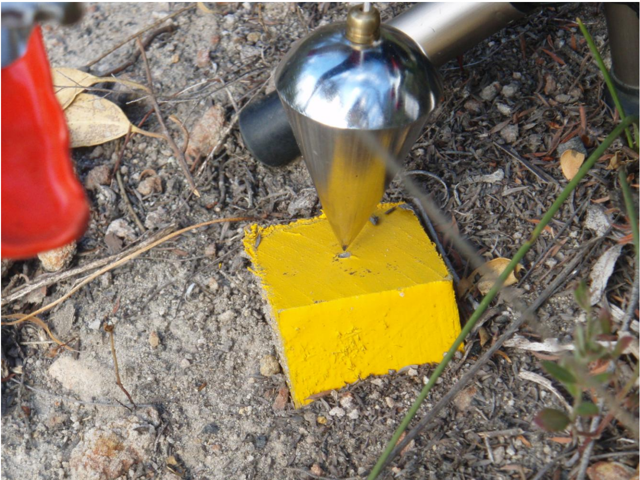
Figure 6 Positioning the plumb bob over a reference peg (TV-6 March 2009)
