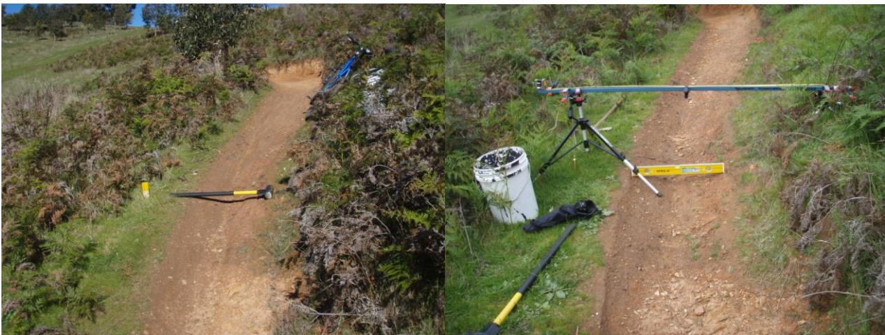
Figure 26 DT-17 in August 2008 and September 2009 showing no change despite the minimal trail to fall line angle. Note the concave tread profile
